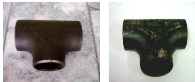
Fig1: 2 inches T- shape tube before and after final cutting
